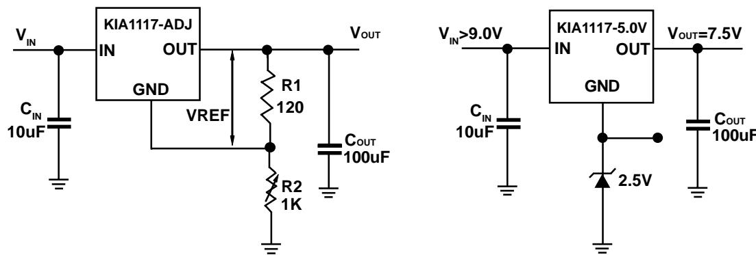
$$V_{OUT} = V_{RE} F \left( 1 + \frac{R2}{R1} \right) + I_{ADJ} R2$$
